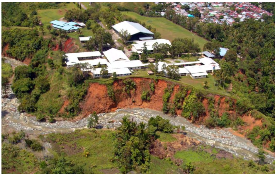
Figure 6. Detail of the primary slip area showing the river eroding the base of the cliff, March 2007. Photo: Tim Harold.
